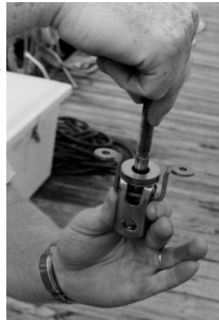
Adding washers to T-bolt
