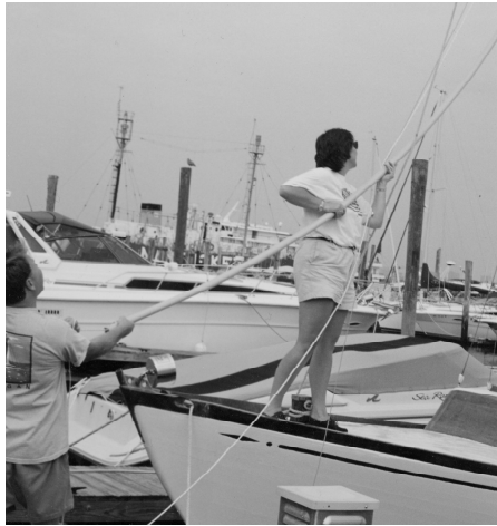
pushing luff extrusion up forestay
