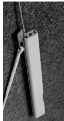
Traveler is opposite sail feed slot (slot is on lower RH side)
