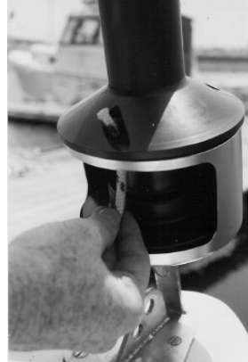
Installing the furling line
