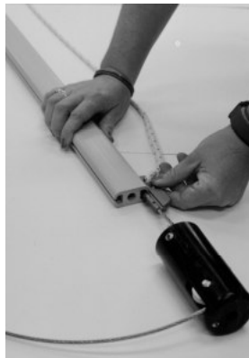
Inserting traveler into luff groove
