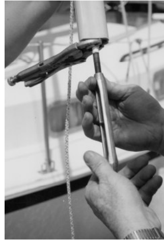
screwing TB on stud
