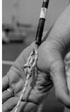
connecting swage stud to messenger line
