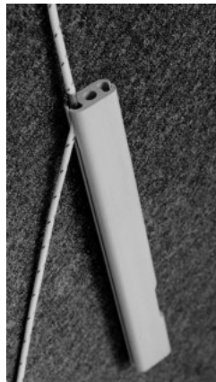
Starting the ferrule down the luff extrusion
