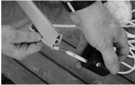
Pull halyard thru HTF. Ferrule gets inserted into the top of the luff extrusion.
