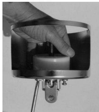
Assembling cup, bearing and antirotation strap
