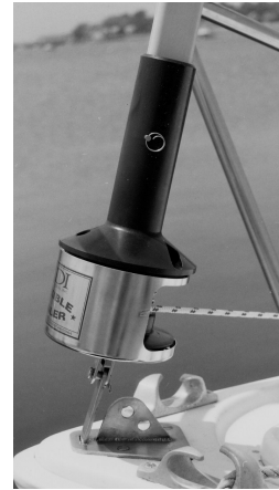
Furler w/ luff support pin installed
