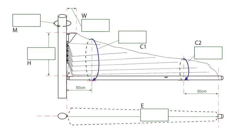
M: Circumference of mast (including accesories such as pole eye, winch, etc.)
