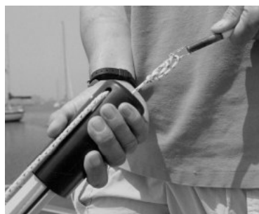
connecting swage stud to messenger line
