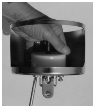
Assembling cup, bearing and antirotation strap
