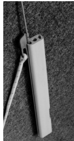
Inserting FF6 traveler into top of luff
