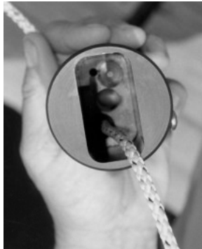
Rope halyard fed into HTF (bottom view)
