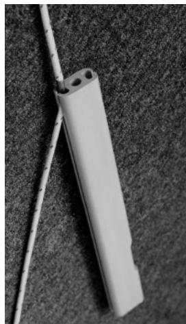
Inserting FF4 ferrule into top of luff
