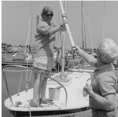
pushing extrusion up forestay
