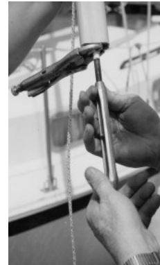
screwing turnbuckle on stud
