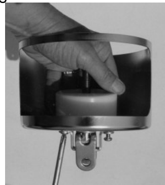
Assembling cup, bearing, and antirotation strap
