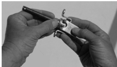
Adding washers to the T-bolt
