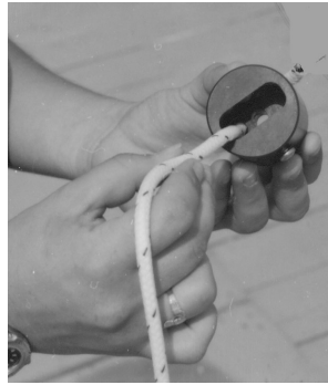
Feed halyard into HTF & out the side. (bottom view)
