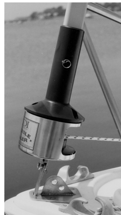
Furler w/ luff support pin installed
